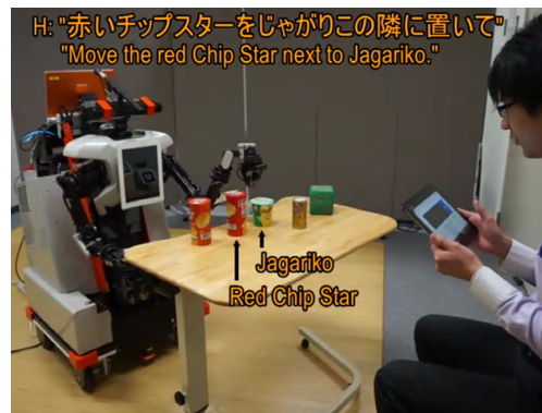
Fig. 1. Sample dialogue using rospeex between a speaker and “Daia,” our robot platform. Large vocabulary continuous speech recognition is possible. In other words, the grammar containing proper nouns such as “Chip Star” and “Jagariko” is not hand-coded.
