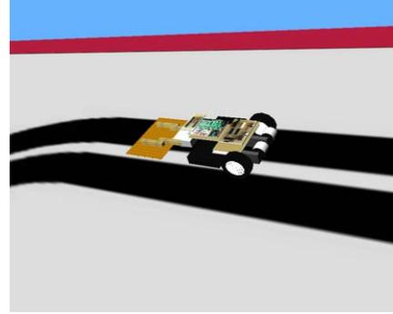
Figure 3. Line-following robot
